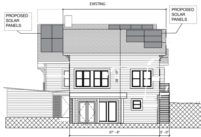
② South Exterior Elevation 1/8" = 1'-0"
