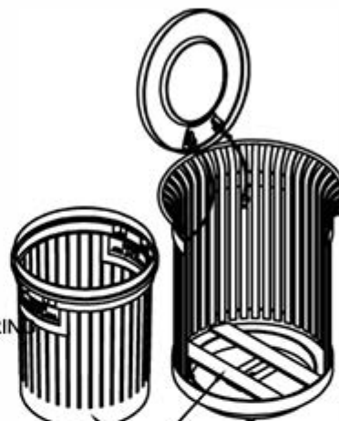
36-GALLON CAPACITY HIGH DENSITY PLASTIC LINER (WEIGHT NOT TO EXCEED 6 LBS.) SITS ON 3/8" x 3" SUPPORT BARS
