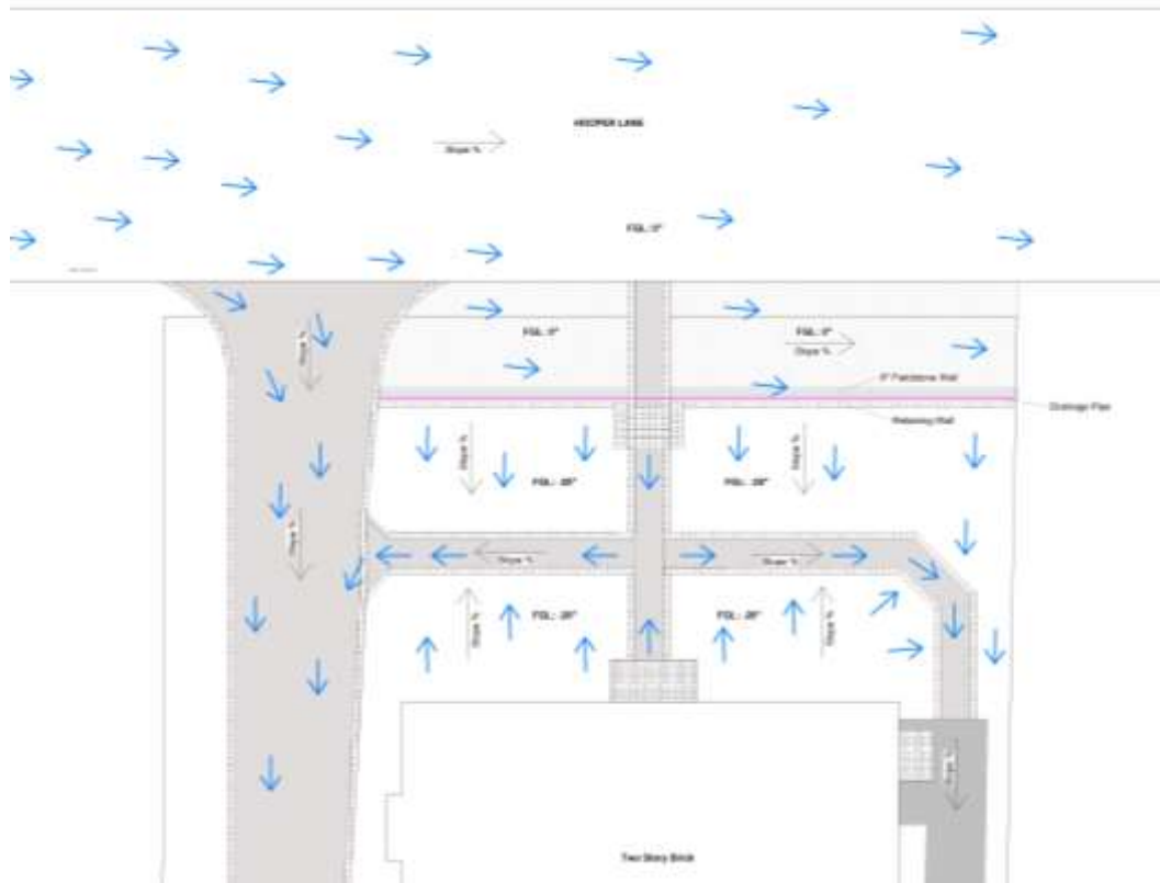
Figure 62 - New Landscape - Stormwater Drainage Diagram
