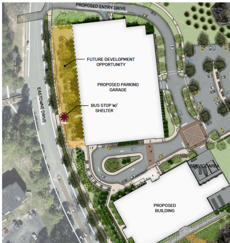
Figure 2. Illustrative site plan showing a) liner building site along western elevation of the parking garage, b) alignment of stair along western end of entry plaza connecting to the bus shelter, and c) street trees in an 8' planter strip between the travelway and sidewalk along Eastowne Drive. (Image from applicant letter, October 16, 2018)
