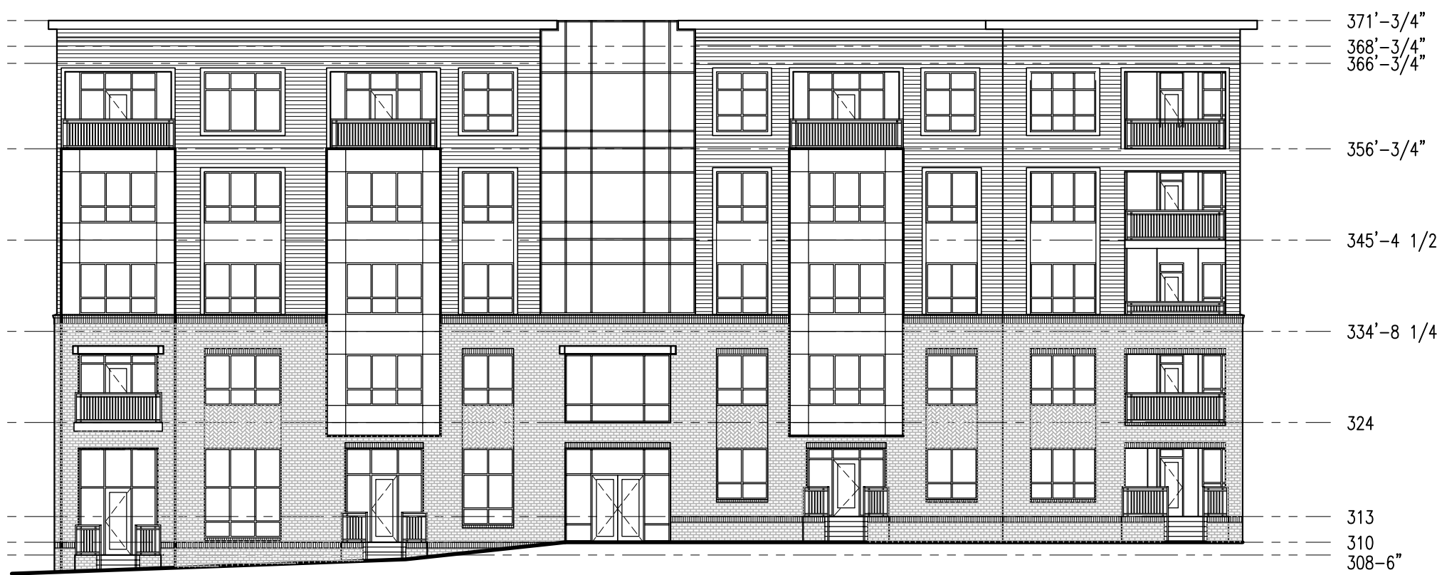
BUILDING 3 ELEVATION B - NOVUS LANE SCALE: 1/16" = 1'-0"
