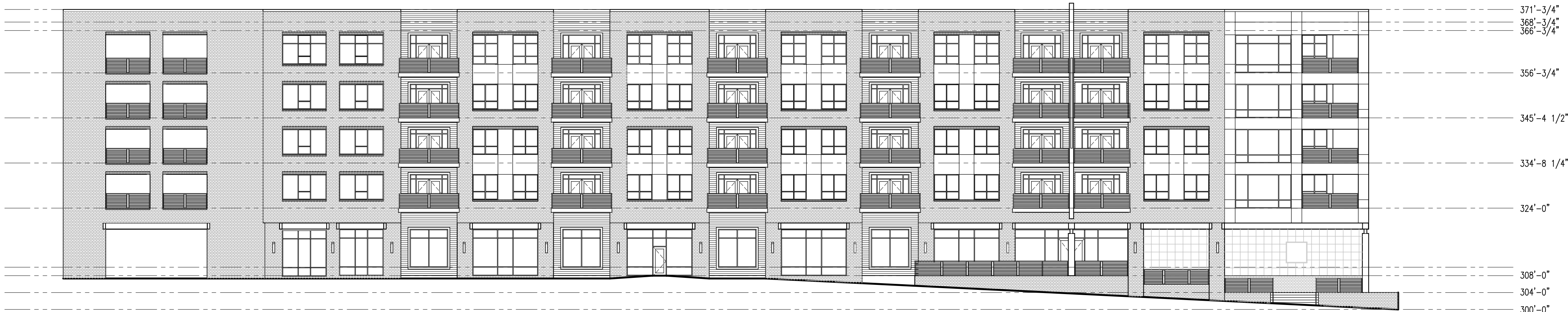
BUILDING 3 ELEVATION - STREET 1 SCALE: 1/16" = 1'-0"
