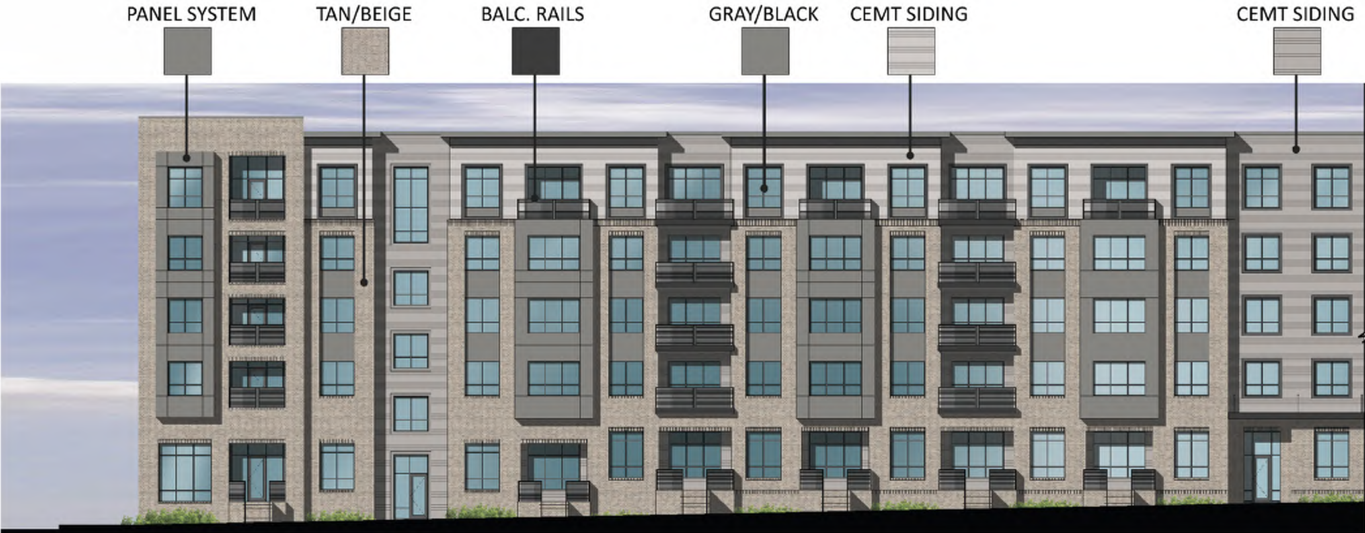
BUILDING 4 ELEVATION - STREET 1 SCALE: 1/16" = 1'-0"
