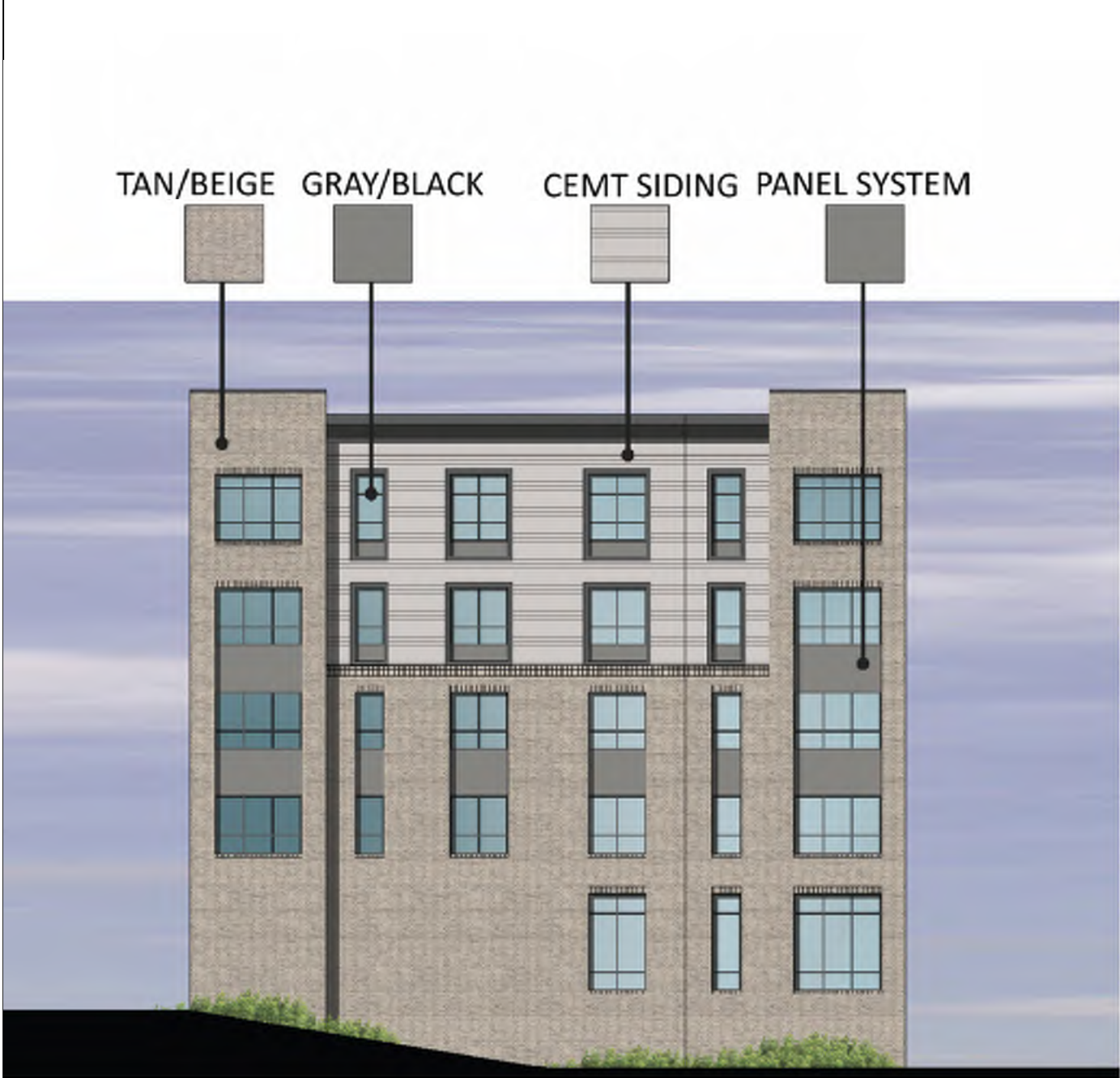
BUILDING 4 ELEVATION - NORTHWEST SCALE: 1/16" = 1'-0"
