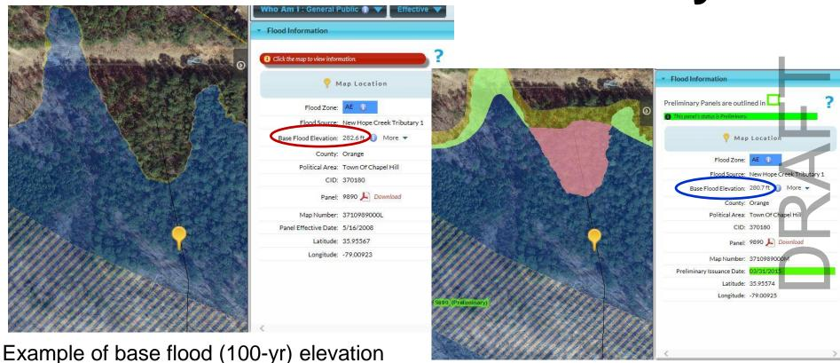
Example of base flood (100-yr) elevation reduction and boundary changes
