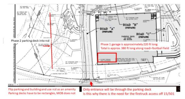
Current Site Plan – Note dotted lines for parking deck expansion into RCD, 380 foot parking deck with only entrance to property through the deck.
