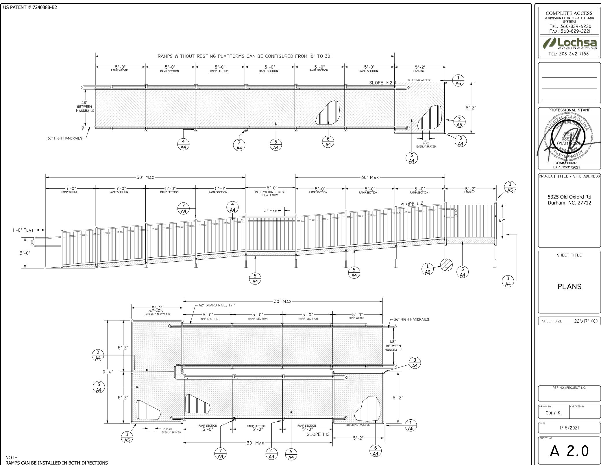
RAMPS CAN BE INSTALLED IN BOTH DIRECTIONS
