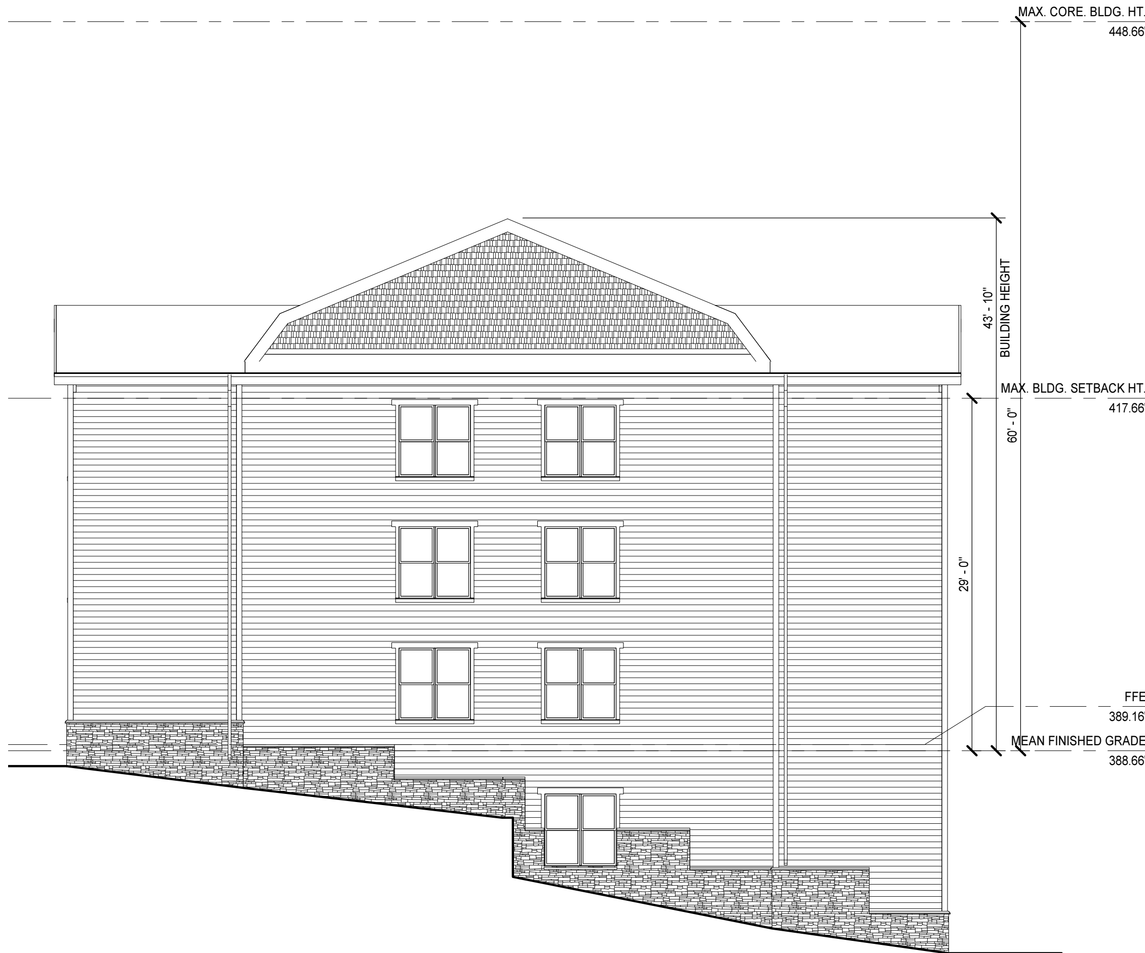
4 EAST ELEVATION - BUILDING B 1/8" = 1'-0"
