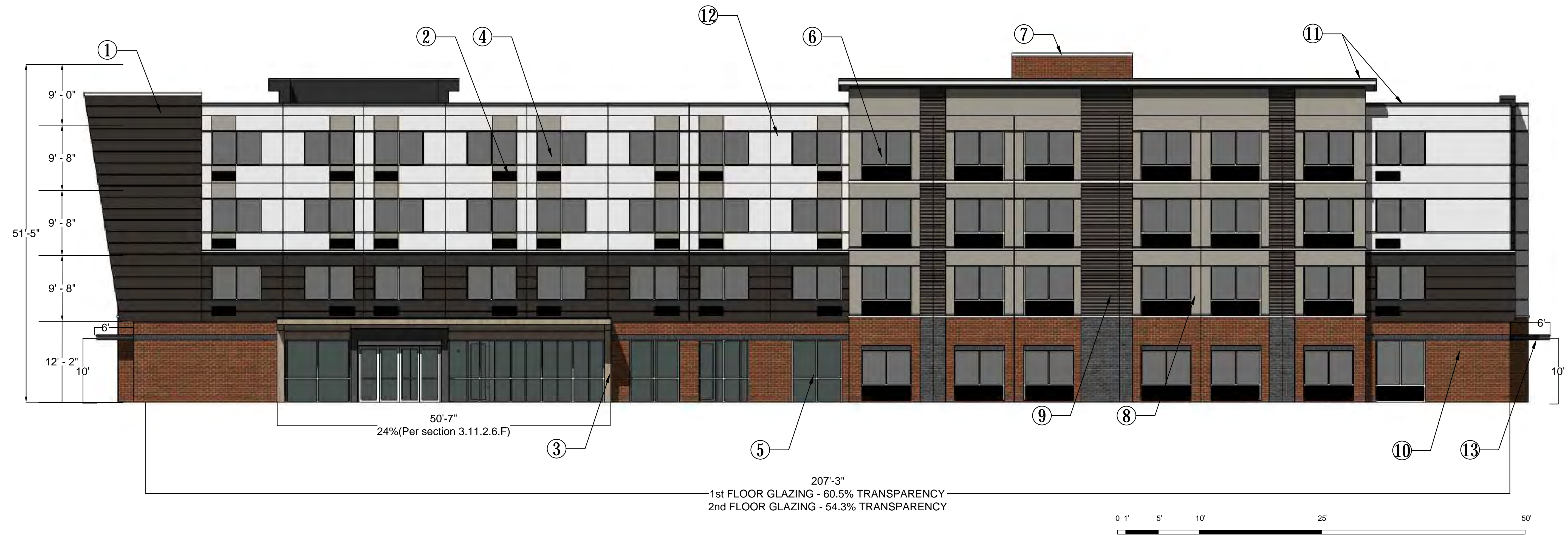
1 FRONT "SOUTH" ELEVATION (ENTRANCE/PARKING/DROP-OFF FACADE) A1 1/4" = 1'-0"
