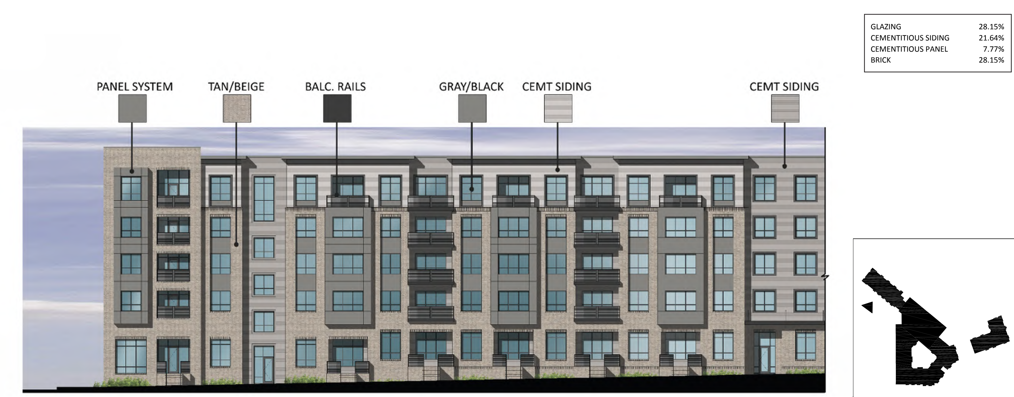
BUILDING 4 ELEVATION - STREET 1 SCALE: 1/16" = 1'-0" 1
