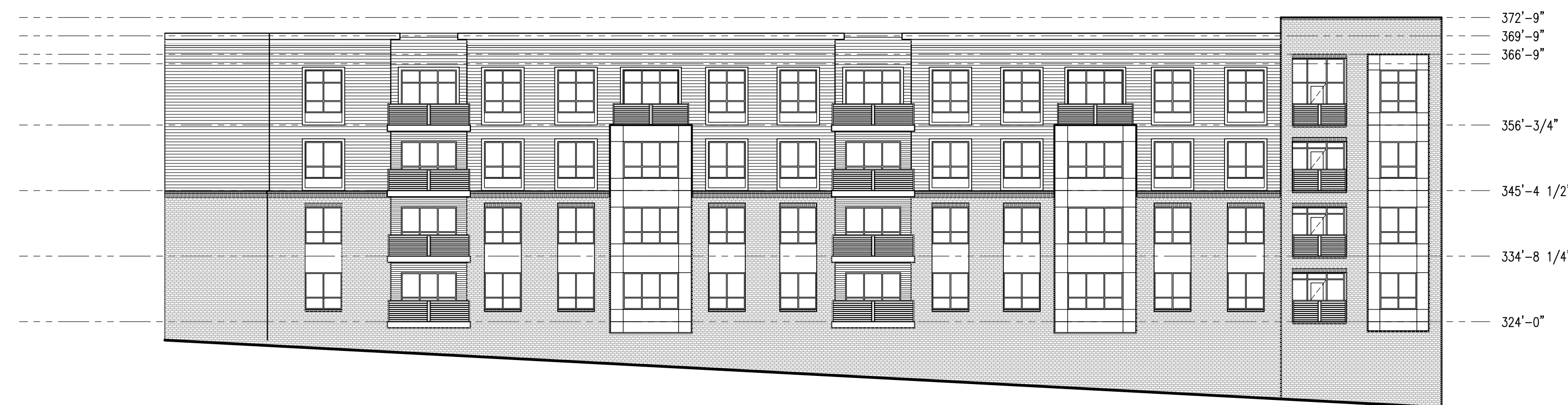
BUILDING 4 ELEVATION - REAR SCALE: 1/16" = 1'-0"
