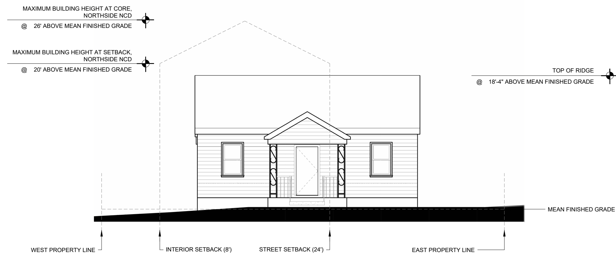
1 EXISTING ELEVATION - SOUTH SCALE: 1/8" = 1'
