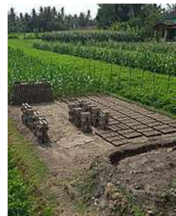
Raw bricks sun-drying before being fired
