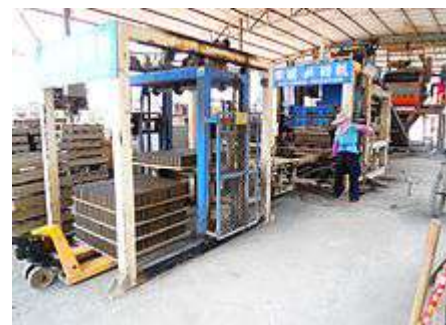
A concrete brick-making assembly line in Guilinyang Town , Hainan, China. This operation produces a pallet containing 42 bricks, approximately every 30 seconds.
