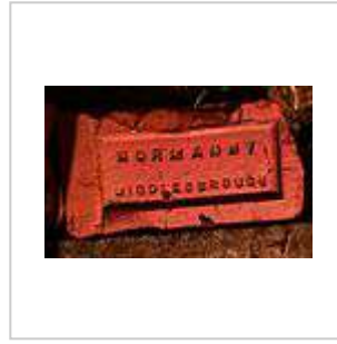
Brick made as a byproduct of ironstone mining Normanby – UK
