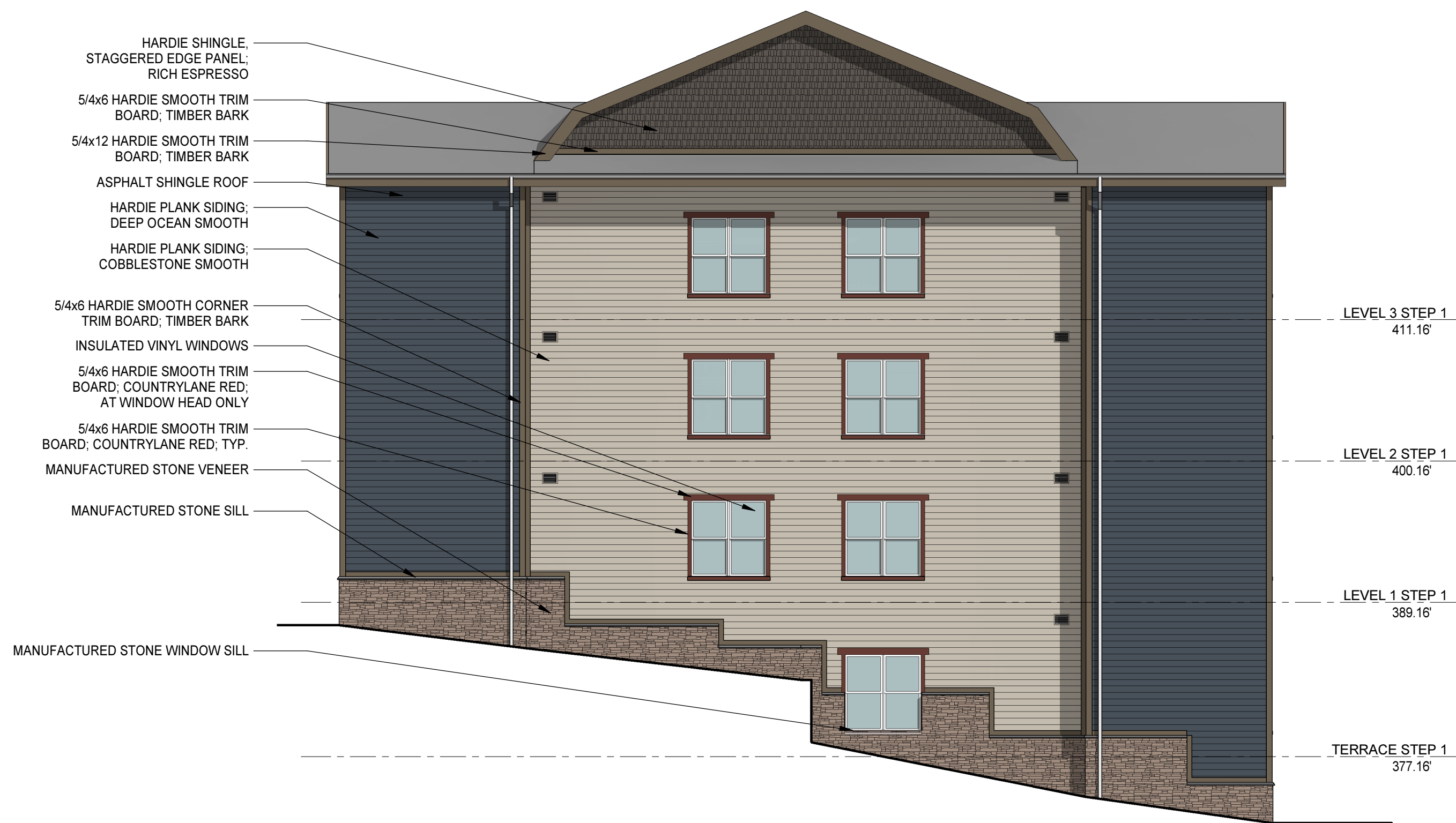
1 EAST ELEVATION - BUILDING B 1/8" = 1'-0"
