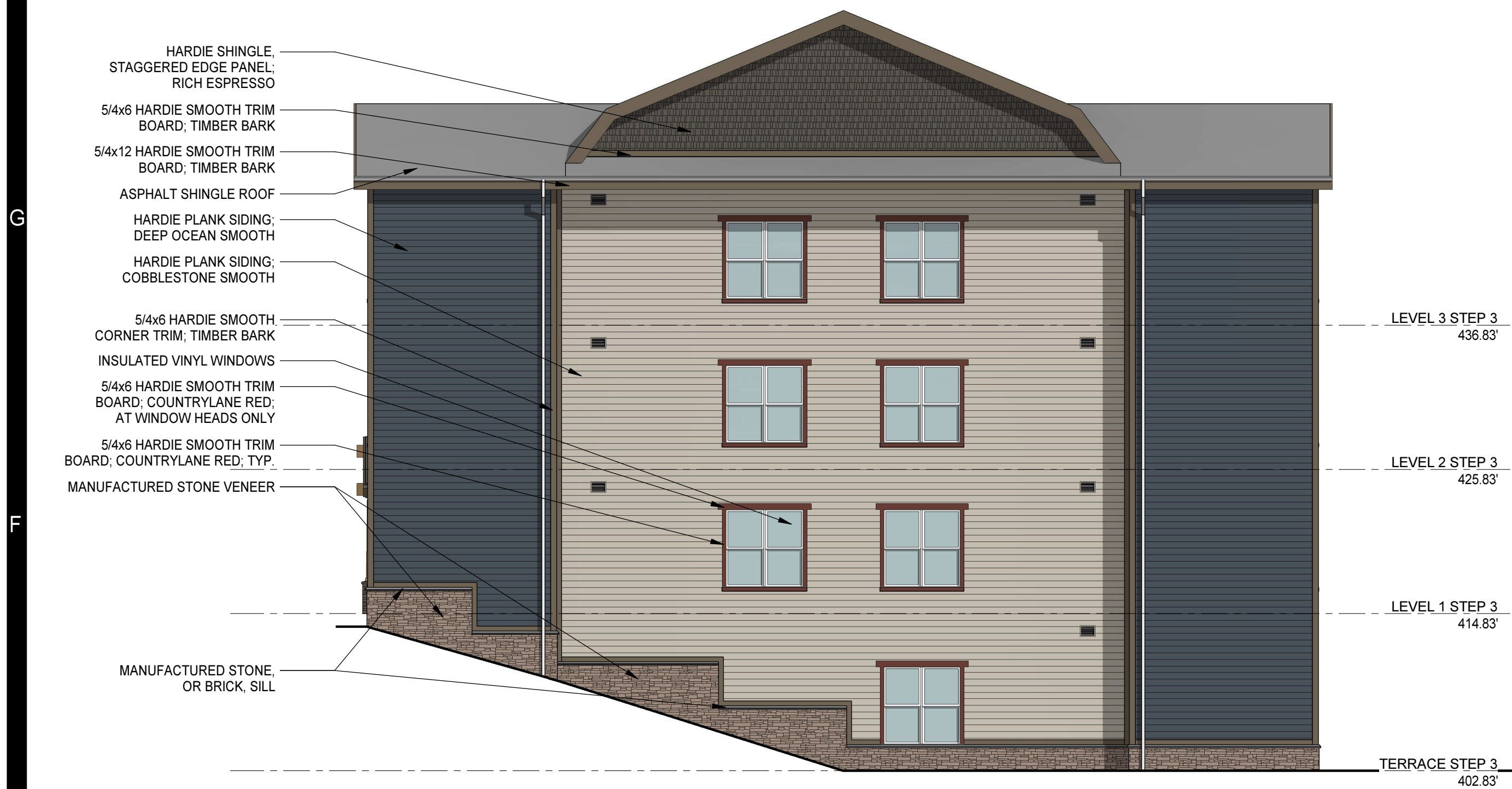
1 EAST ELEVATION - BUILDING A 1/8" = 1'-0"
