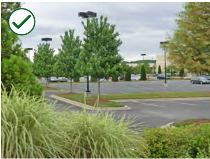
Figure 3-33 Divide a large parking area into interconnected, small modules with landscape buffers.
