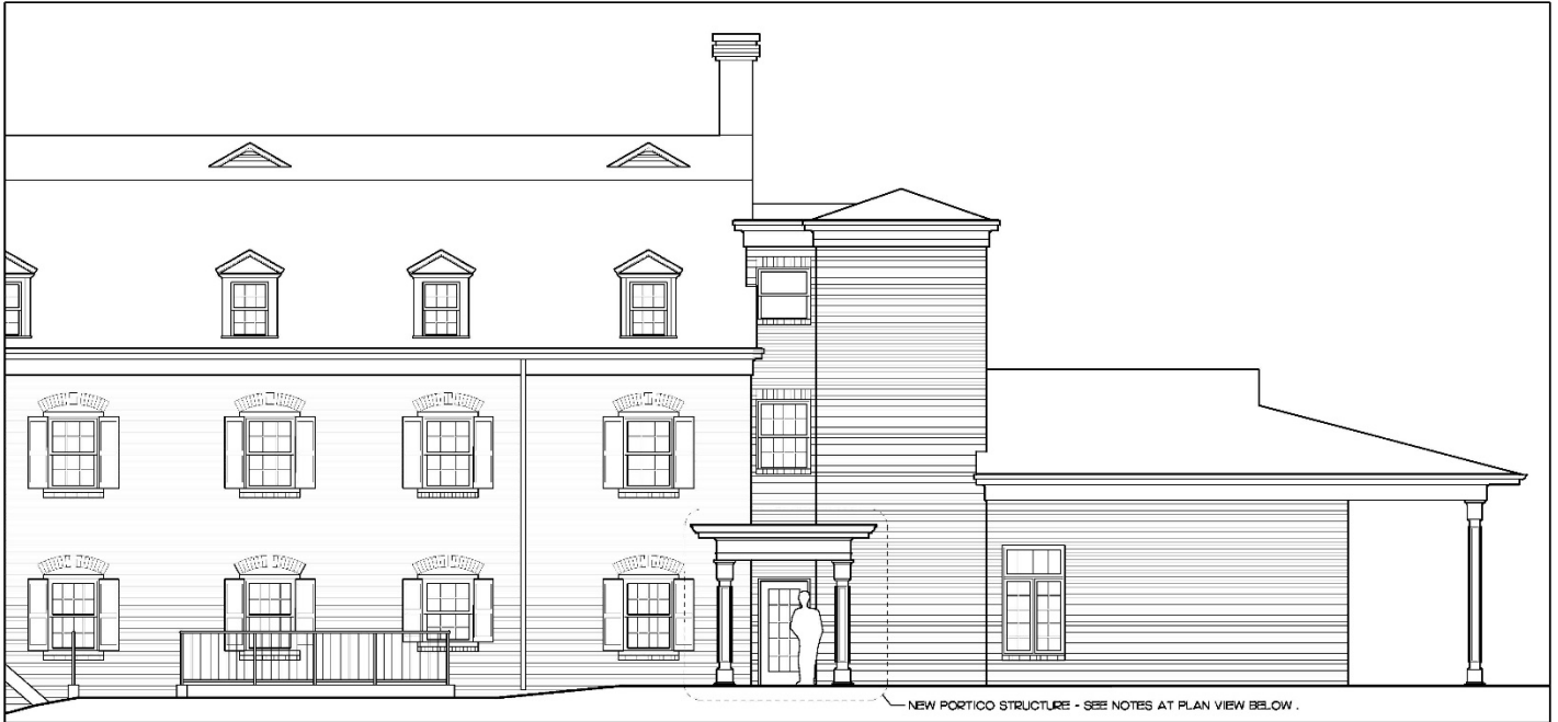
PARTIAL WEST ELEVATION • NEW ENTRY PORTICO SCALE: 1/4" = 1'-0"
