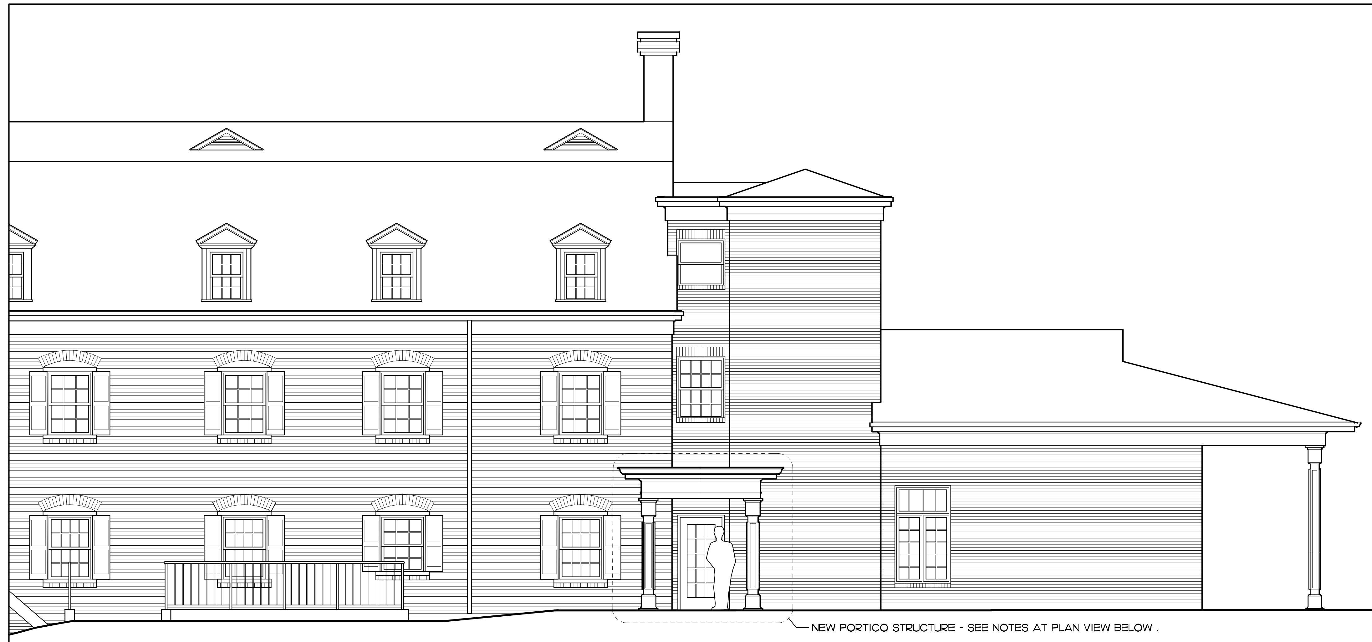
1 PARTIAL WEST ELEVATION • NEW ENTRY PORTICO SCALE: 1/4" = 1'-0"
