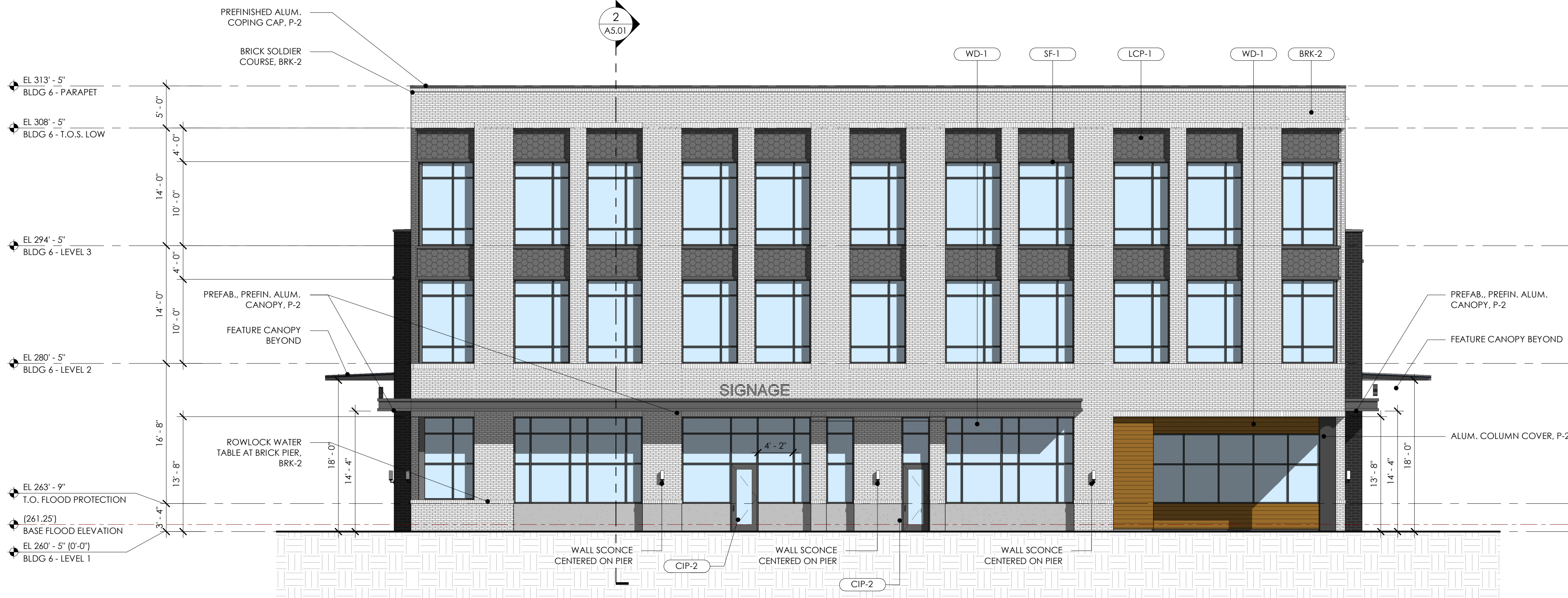
2 A4.02 BLDG 6 - NORTH ELEVATION SCALE: 1/8" = 1'-0"
