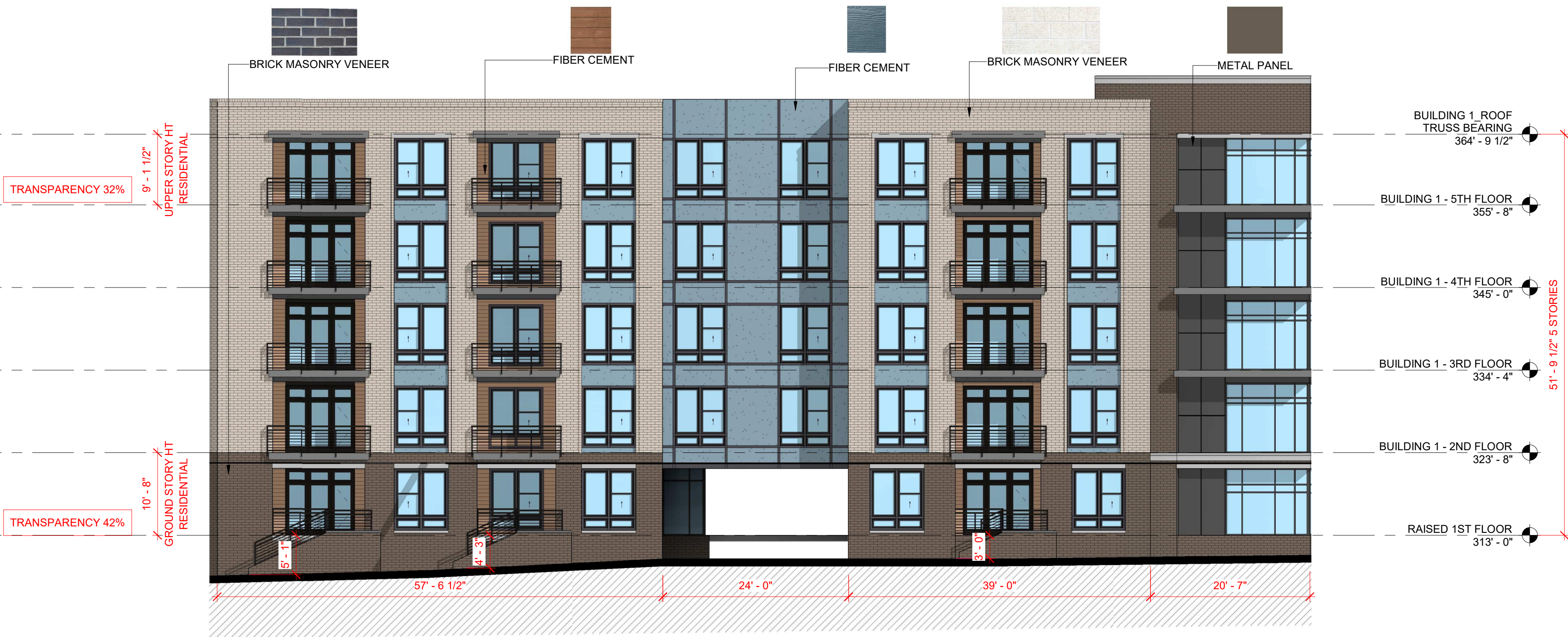
BUILDING 3 - ELEVATION - NOVUS LANE 2 3/32" = 1'-0"
