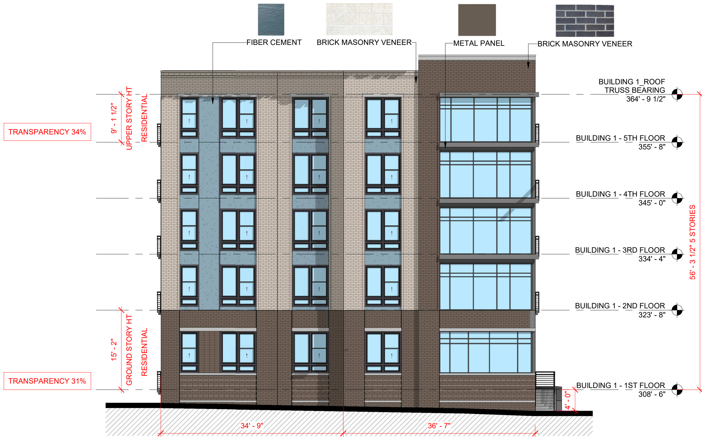
BUILDING 4 - ELEVATION - NORTHWEST 2 3/32" = 1'-0"
