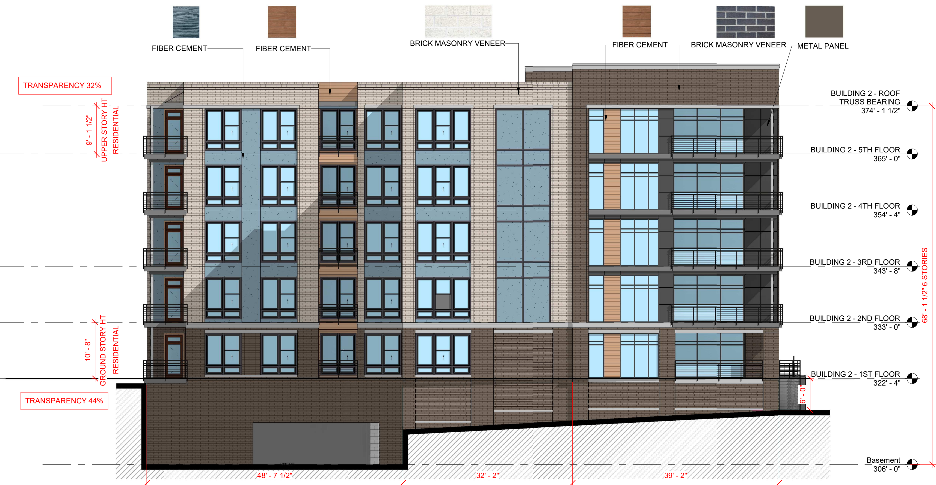
BUILDING ELEVATION - STREET B 4 3/32" = 1'-0"
