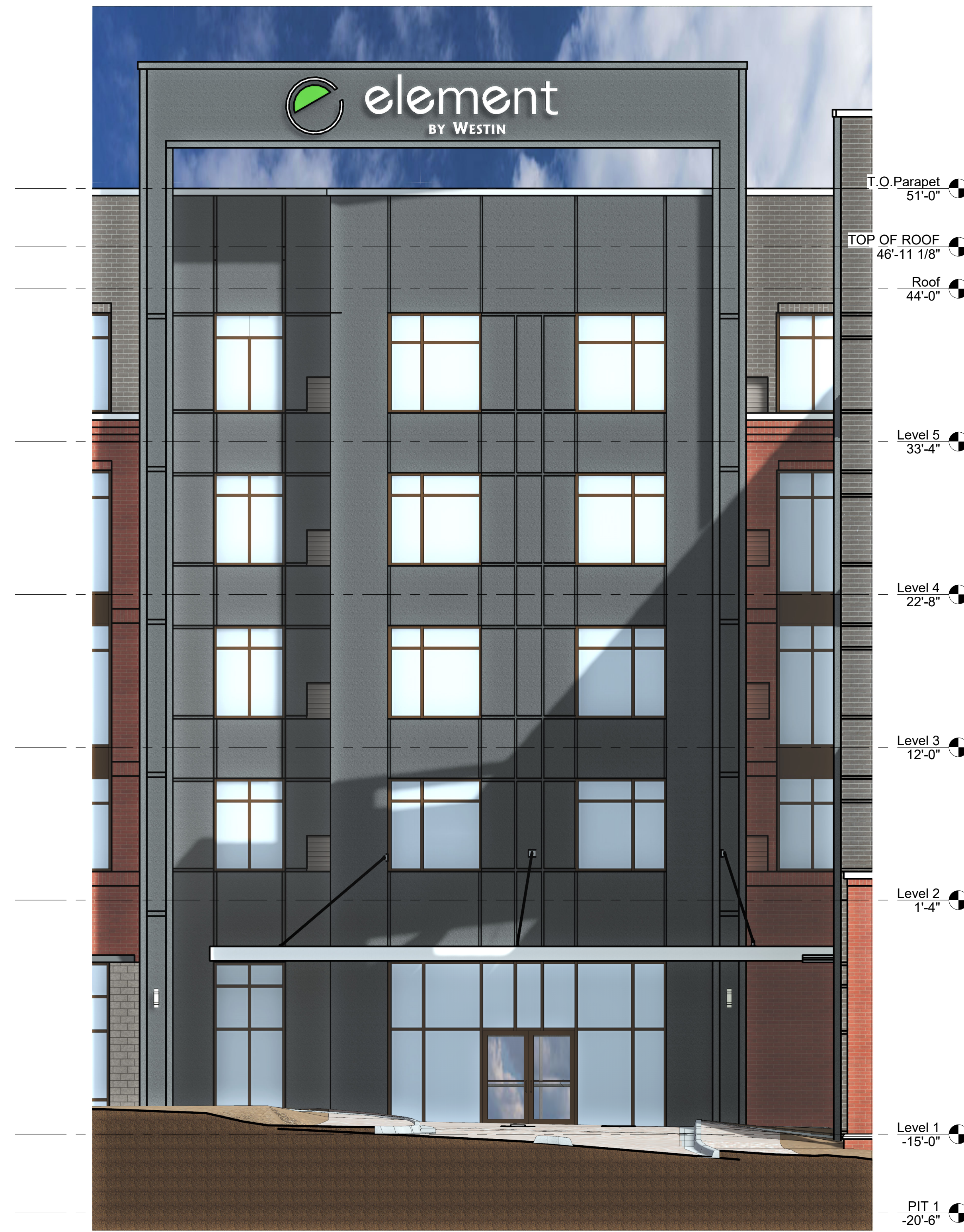
1 ELEVATION - EAST BRAND WALL Scale: 3/16" = 1'-0"
