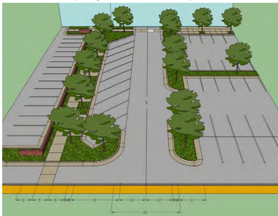
45 ° Angled parking - parking bays
