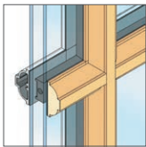
OGEE INTEGRAL LIGHT TECHNOLOGY 1 7/8", 1-1/4" OR 2"
