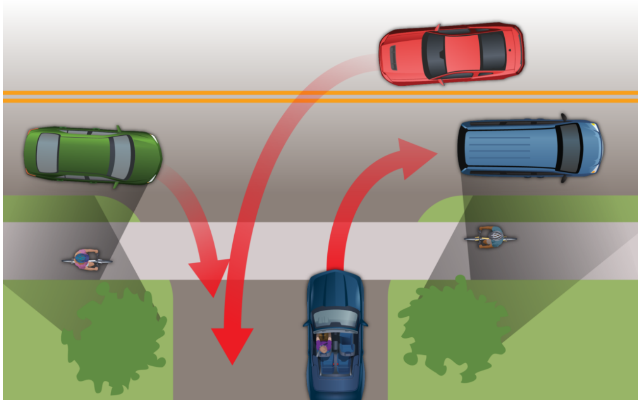
Cycling Savvy 4 graphic depicting common sidepath crash mechanisms: Left Cross, Right Hook, and DriveOut . Estes Drive would add pedestrians and a separate Sidebike to this scenario.
