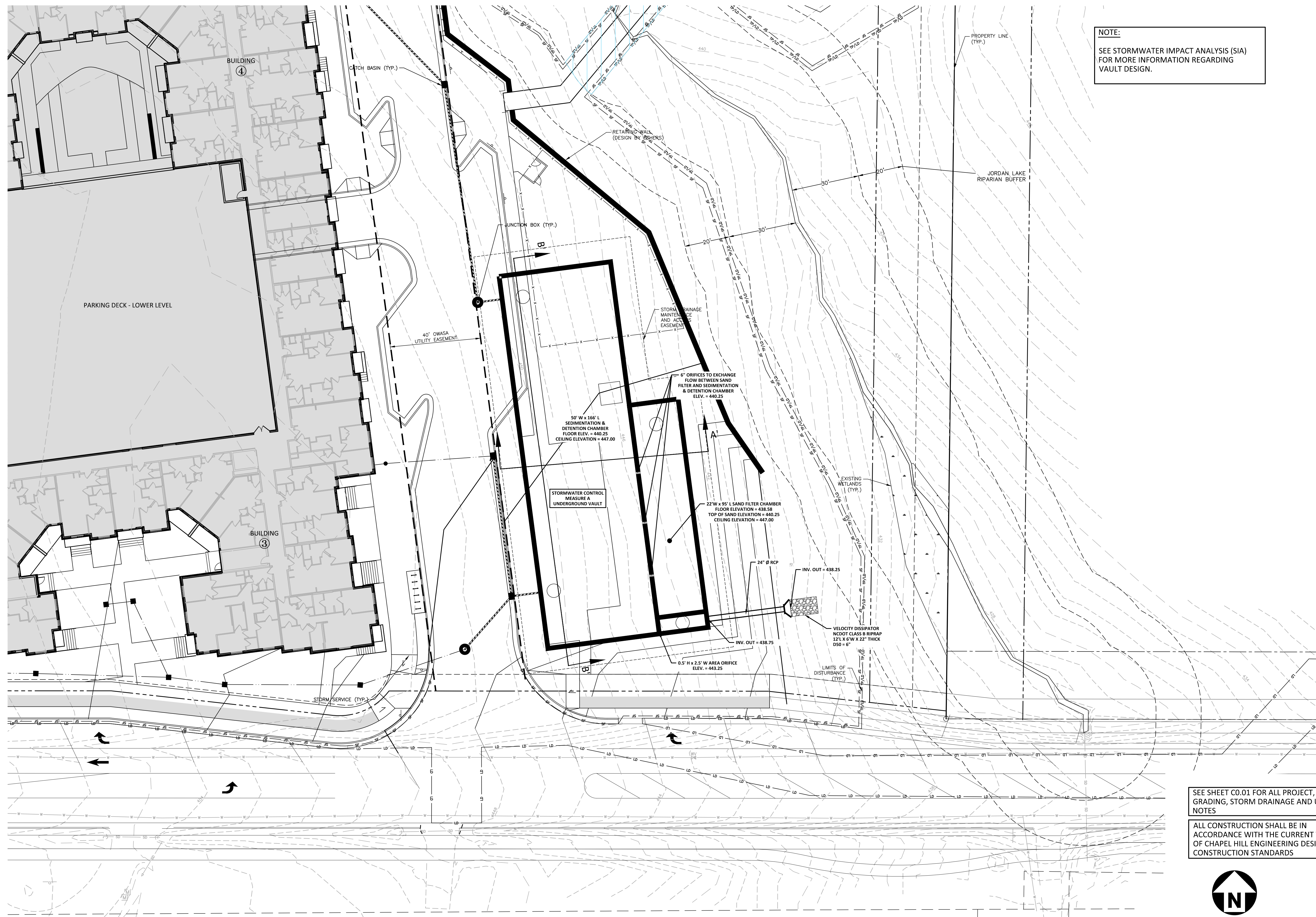
UNDERGROUND SAND FILTER & DETENTION SYSTEM 'A' PLAN VIEW 1" = 20'
