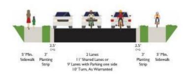
27 between Back-of-Curb sections (Min Width) Includes Parking, Curb, and Gutter.
