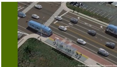
Dedicated Curb Lane - Construct a New Lane
