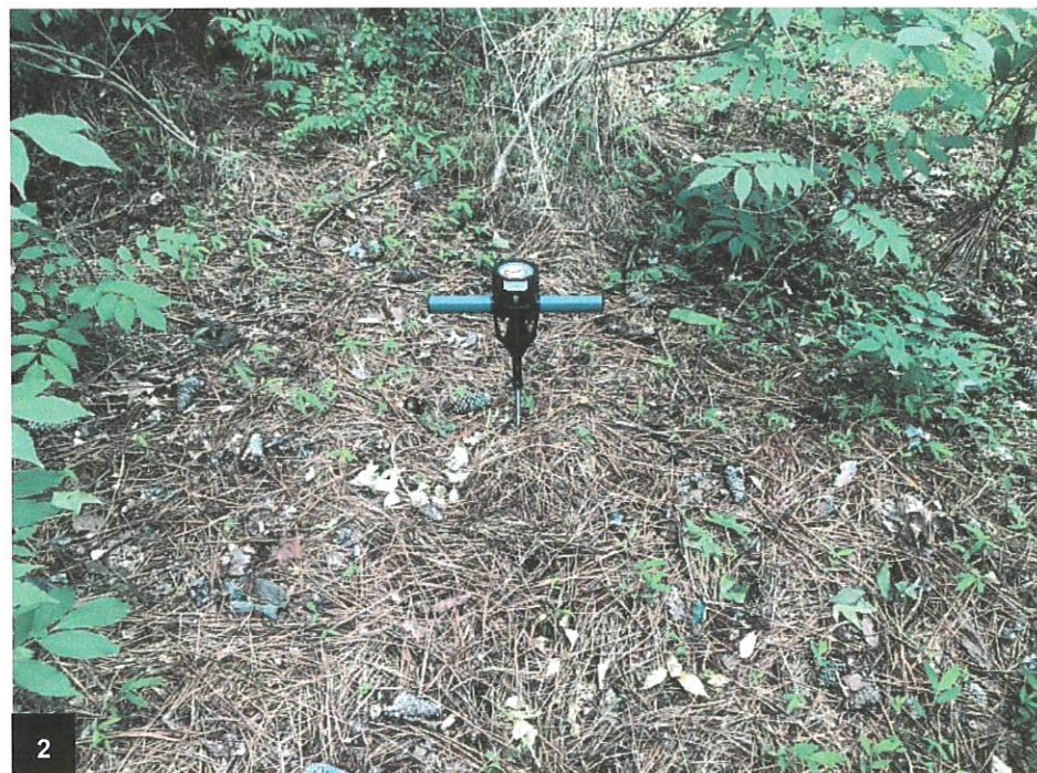
Probe rod in unsuitable soils
