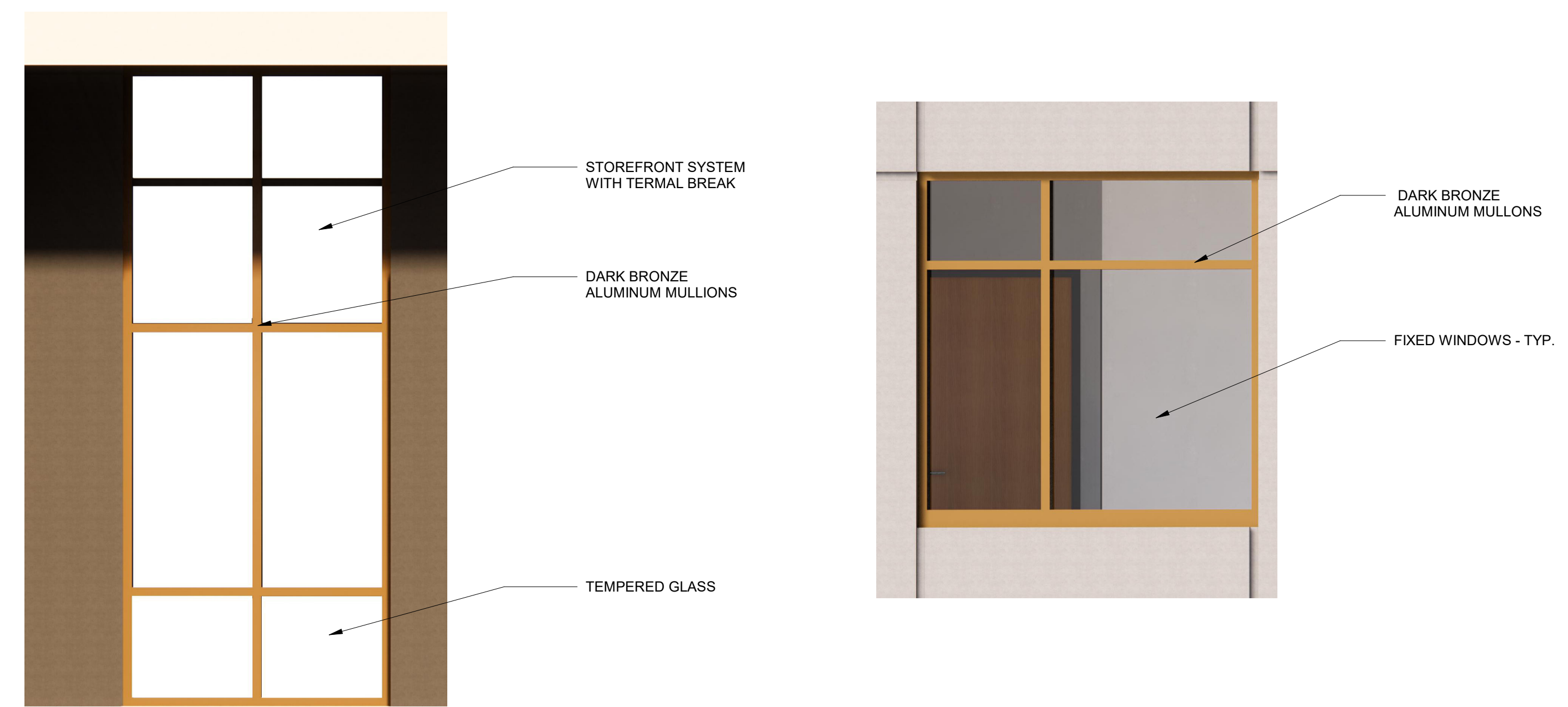
4 Typical Storefront @ Metallic Coating Scale: 1/2" = 1'-0"
