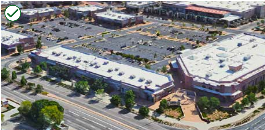
Figure 3-32 Locate a surface parking lot so it will minimize gaps in the continuous building wall of a commercial block.
