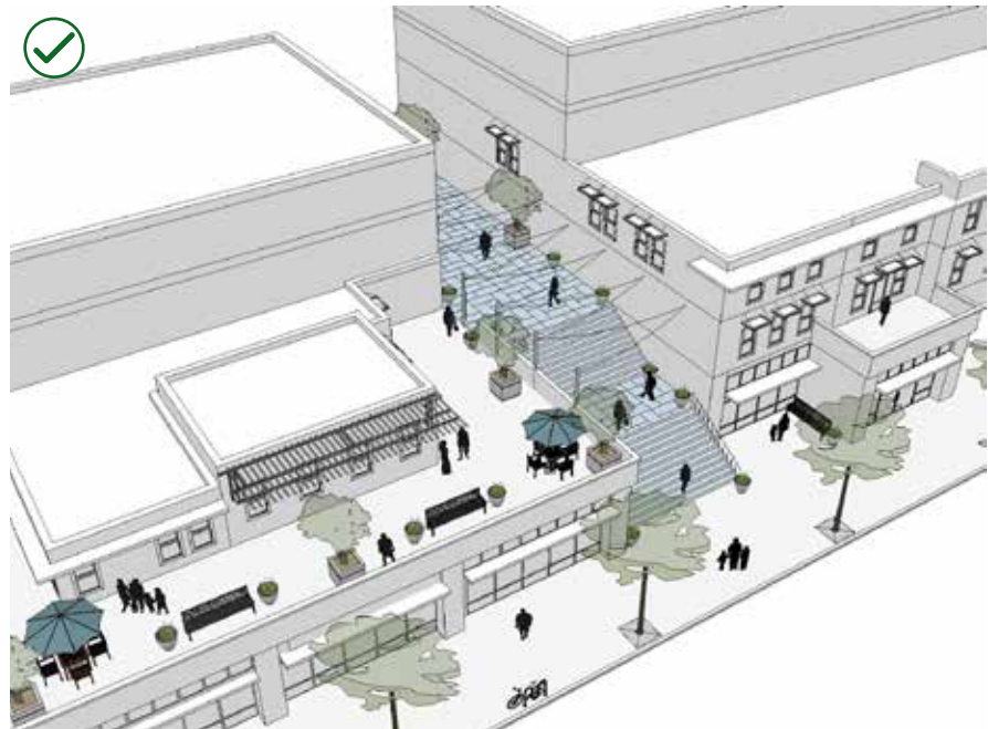
Figure 3-25 Design a rooftop outdoor amenity space to be highly visible and easily accessible from the public way. The stairs and elevator should be exterior or located in a vestibule.
