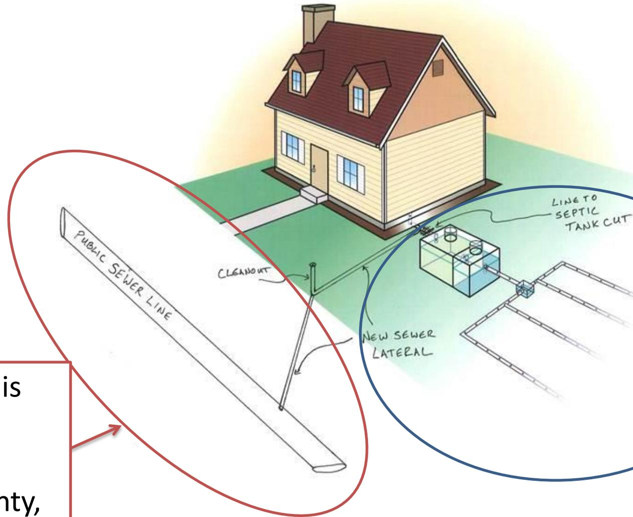
Onsite plumbing within the property lines includes the sewer laterals. Note the abandonment of the septic tank and drain field
