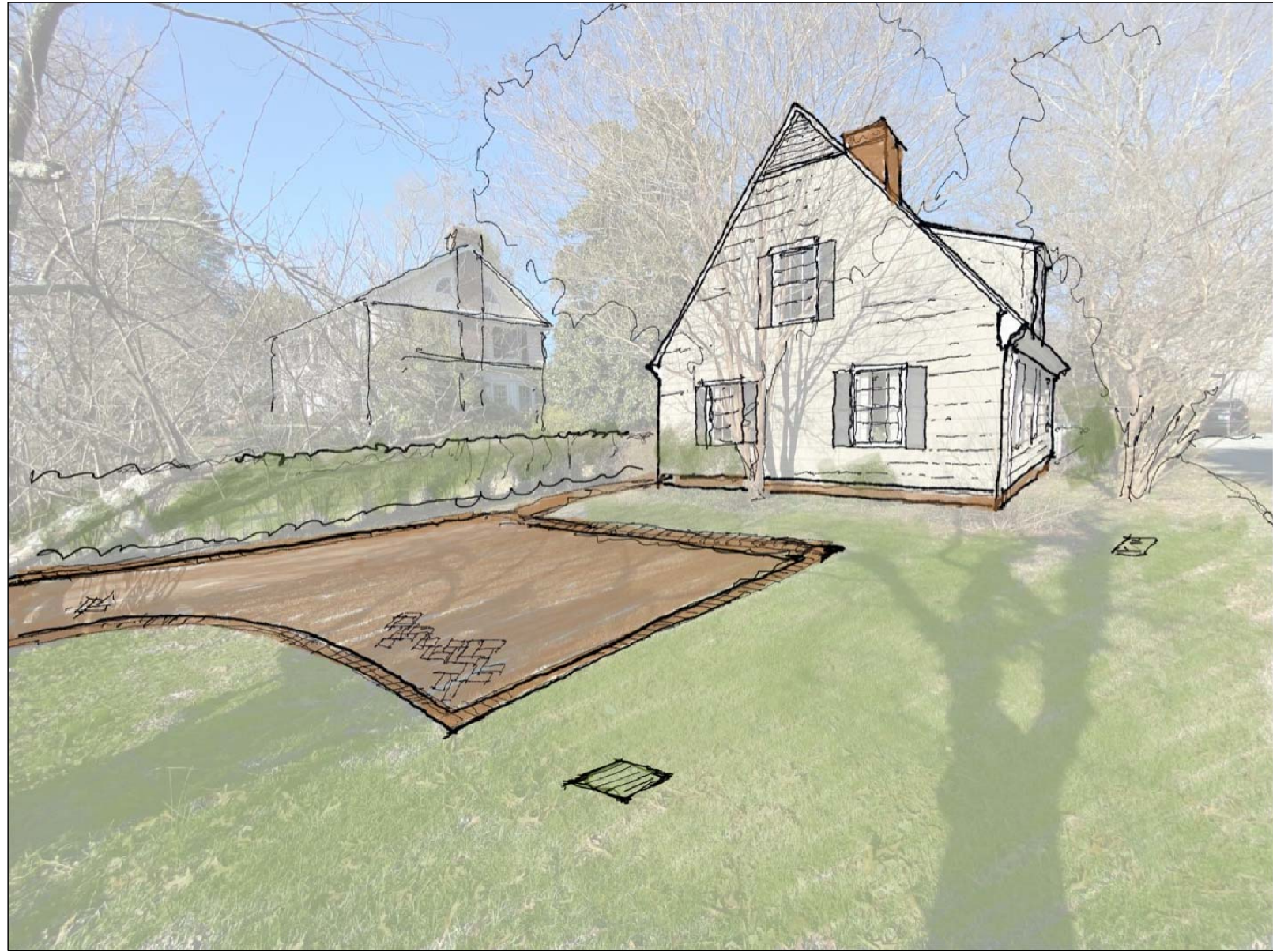
Sketch of proposed Brick Parking Court (permeable brick pavers bordered with Bullnose brick curb) NOTE: parking is 18 ft. wide to accomodate two cars
