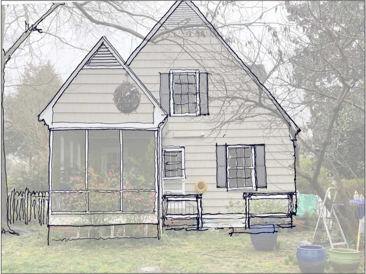
Sketch of the proposed rear deck, using treated decking boards and white wooden posts with a 2x4 wooden cap rail. Existing screen porch and door to remain.
