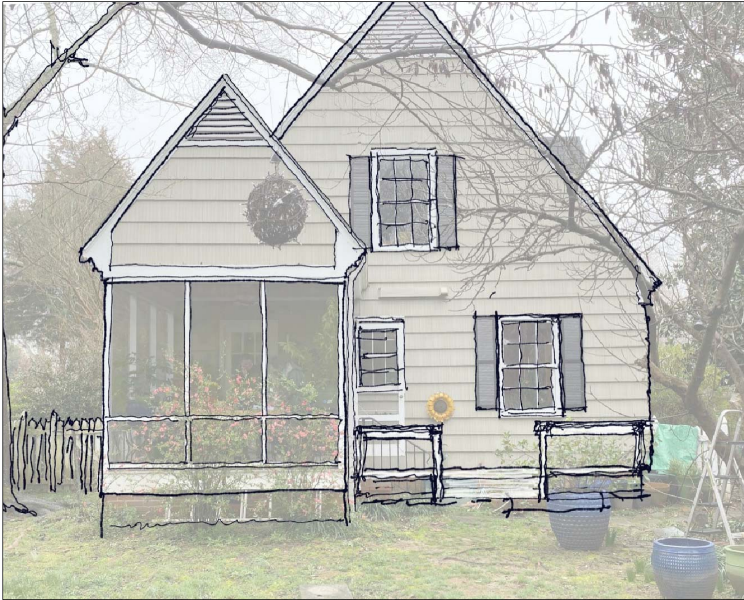
Rear Elevation of Deck with simple Wood Posts and Railing Cap and Step Railing Detail NOTE: The deck will be lower than 30" and railing is not required, but the railing is preferred to provide space.
