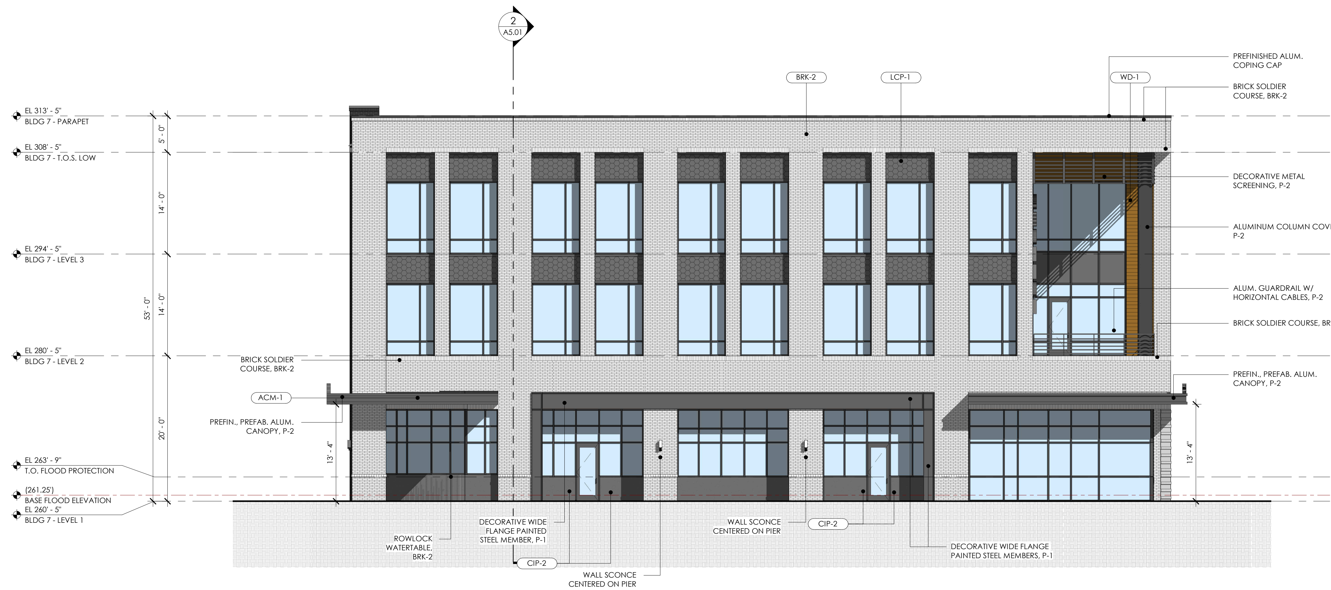
2 BLDG 7 - NORTH ELEVATION A4.02 SCALE: 1/8" = 1'-0"
