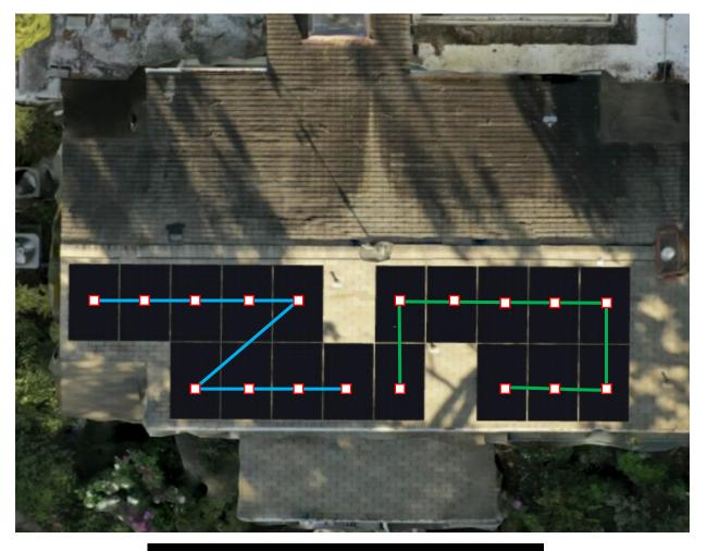
Module: 405W Q.Cell Q.Peak Duo G10+ ■ Optimizer: SolarEdge S440
