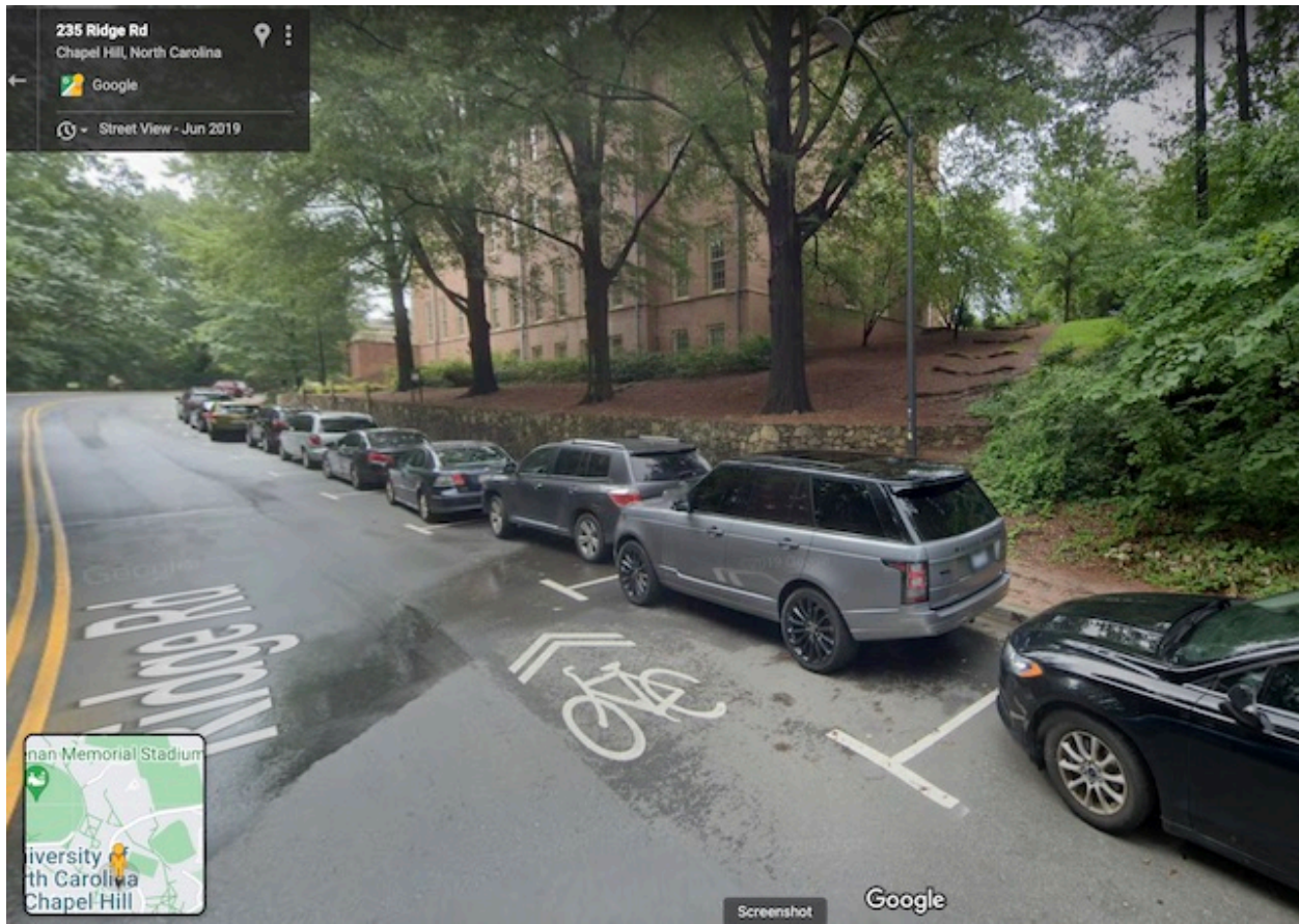
Image 4. Shared Lane Marking in the Door Zone on Ridge Road.
