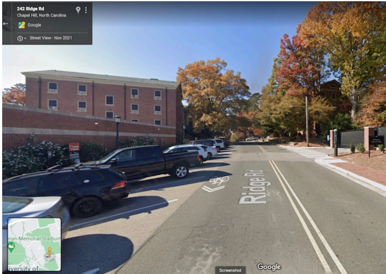
Image 5. Shared Lane Marking placed too close behind angled parking on Ridge Road.
