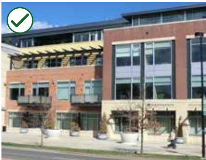
Figure 4-16 Use materials to convey a sense of human scale and visual interest to pedestrians.
