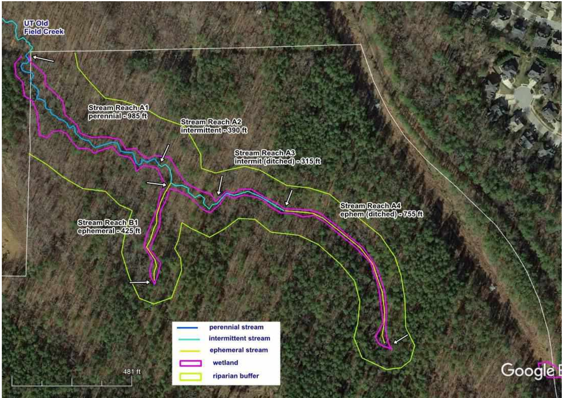
Figure 8A. Streams, wetlands, and regulated buffers, northern section, Old Field Creek watershed. Stream transition points from Town of Chapel Hill.
