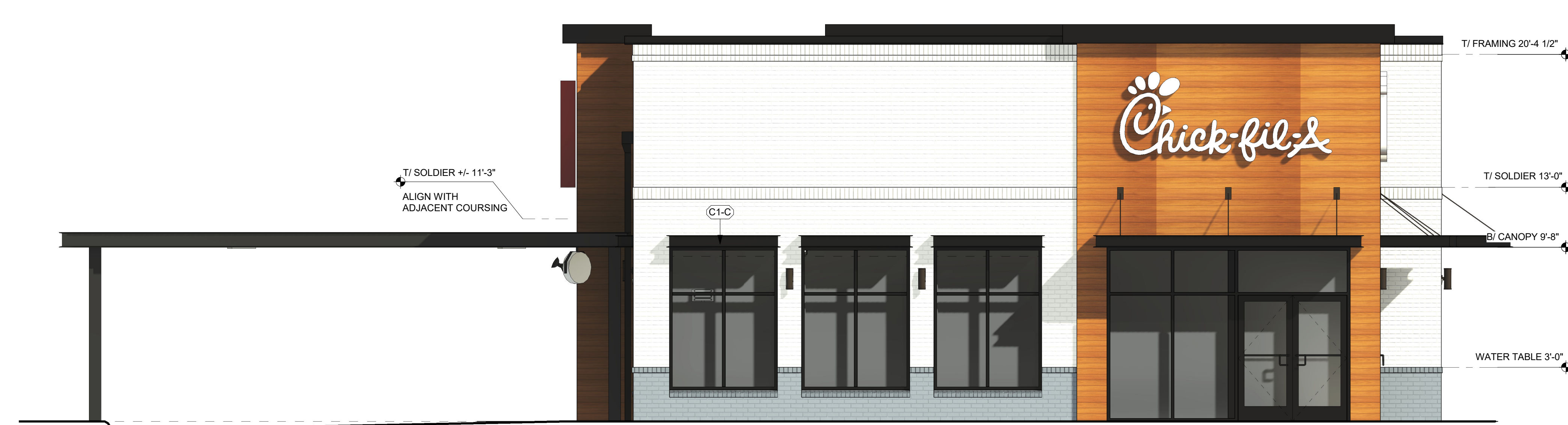
B4 EXTERIOR ELEVATION - SOUTH 1/4" = 1'-0"
