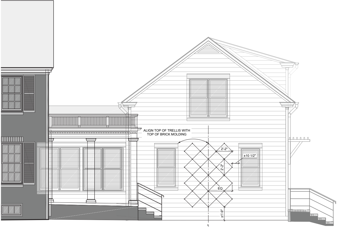
1 STAINLESS STEEL TRELLIS SCALE: 1/4" = 1'-0"
